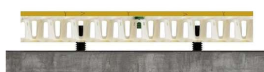
example/section of the CircoFloor system
