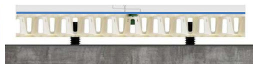
example/section of the CircoFloor system
