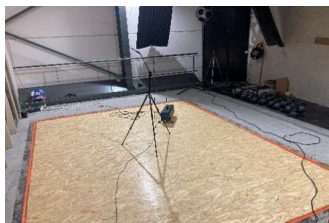
Measurements: four tapping machine positions on the test floor
