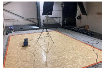
Measurements: four tapping machine positions on the test floor
