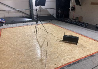
perimeter joint sealed with Perennator
