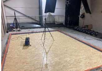
Measurements: four tapping machine positions on the test floor
