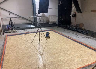
Measurements: four tapping machine positions on the test floor
