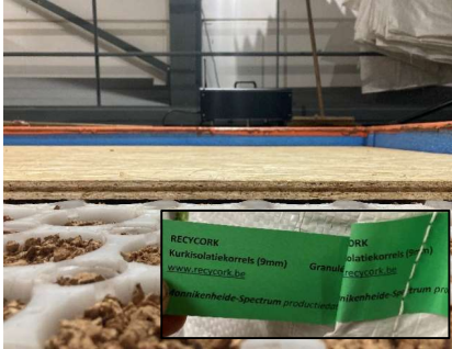
Infill material: Recycork 9 mm
