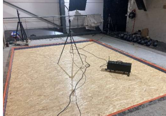
perimeter joint sealed with Perennator
