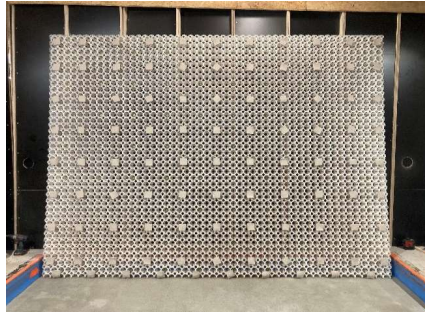
Backside of the full CircoFloor structure (12m²) with 98 supports + pads
